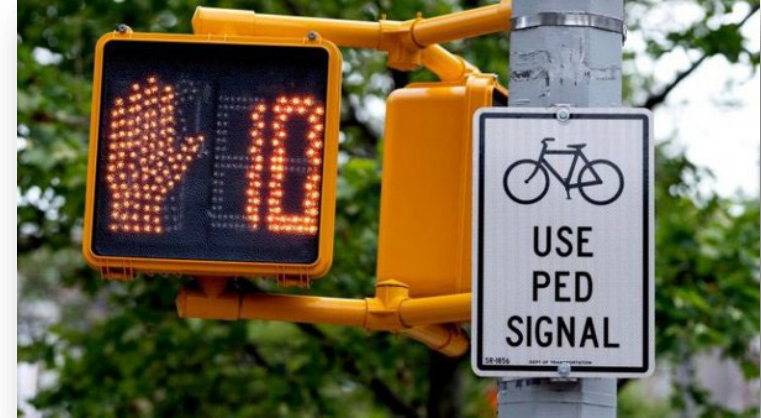
SI18PB- Install pedestrian countdown signal heads
